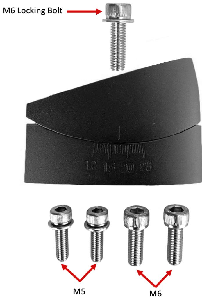
**IMPORTANT:** Apply medium strength thread lock compound (e.g. Loctite 243 blue) to bolt threads before installation. Check the condition of bolts regularly and replace if there are any signs of corrosion or damage.
