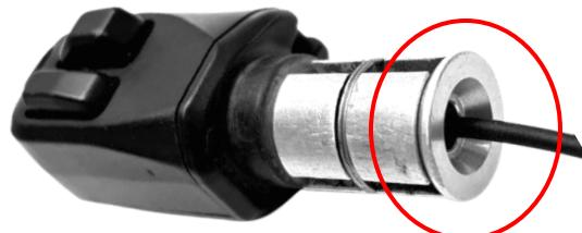
For installing on FastTT aero bars, the shifter cable needs to exit through the centre aluminium barrel.
