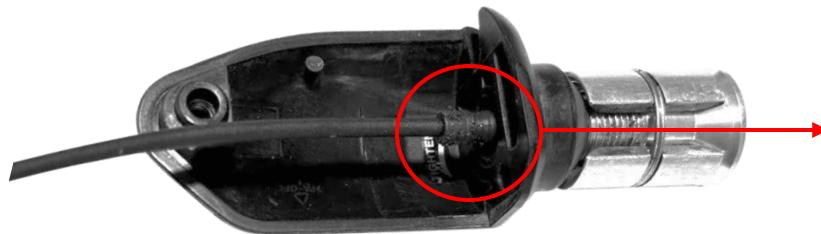
Insert the connector end of the shifter cable through the centre aluminium barrel.
