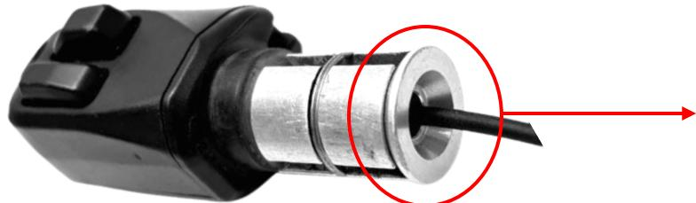
The shifter cable should now exit through the centre aluminium barrel. The shifter cable will insert into the round bar end tube of the aero bars.
