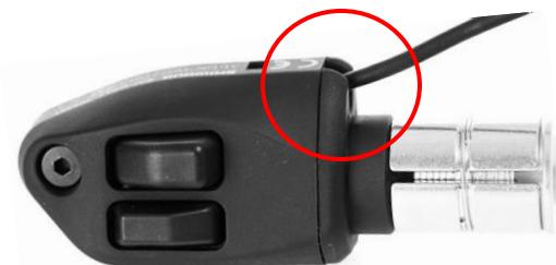
The older model Di2 has the shifter cable exiting the shifter housing on the side.
